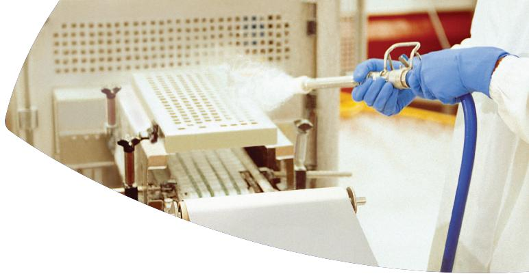
It enables both rinsing, foam application and disinfection covering a large area.
